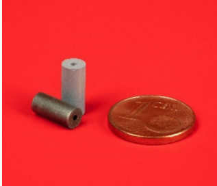
Sintered hollow cathodes made of C12A7 before (white) and after (black) activation.
